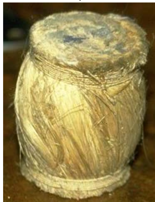
Figure 12. One of the twisted-jute polarizers used by Bose.
