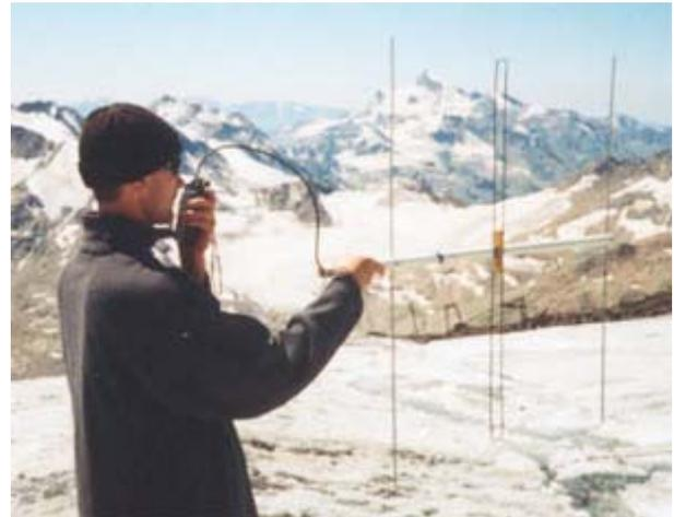
**Figure 1** shows the design of the antenna. Antenna boom is made of a plastic water pipe of 1000-mm of length and of 22-mm OD. Antenna reflector and vibrator both are made of aluminum wire of 5-mm of diameter. Antenna vibrator is made of bimetallic wire of 5-mm of diameter. The vibrator is soldered to PC –board that is the central insulator for the vibrator.
