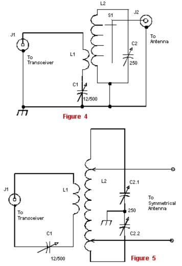
Fig. 4 shows such MU with asymmetrical output, Fig. 5 shows Classical Matching Unit with taps with symmetrical output. These schemes (Fig. 4 and 5) cannot give such careful matching, as shown in Fig. 2 or Fig. 3 have provided. But in case if it is need to minimize dimensions of an ATU the schemes can be used.
