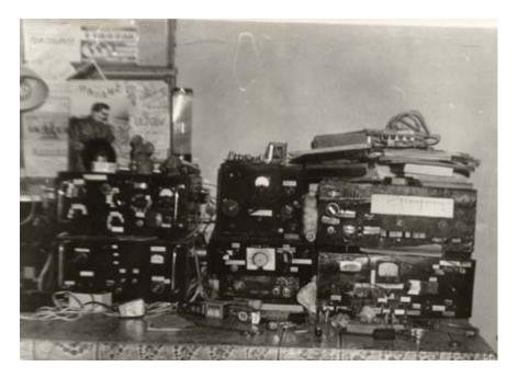
Station UA3ZNW at middle 1980s. Left corner: CW Transceiver and PA for 160, 80, 40, 20 Right corner: PSU 0-16 VDC, 0- 24 VDC, 250- 500 VDC, 6.3 VAC, 12.6 VAC Receiver for 10 meters Center: Automatic key, transmitter for 10 meters, receiver for 160, 80, 40 and 20 meters. AM transmitter for 160 meters. All equipment are home brew
