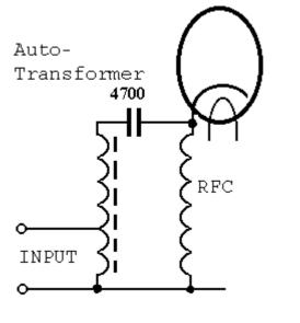
**Figure 1 Matching Autotransformer**
