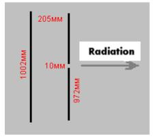
Design of the antenna is very simple. Personally I have made the antenna in 40 minutes. Antenna consists from reflector (length 1002-millimeters) and vibrator (length 972- millimeters, gap for coaxial cable- 10millimeters). Distance between reflector and vibrator is approximately 204 – 210- millimeters. Antennas parts are made from insulated wire in diameter 4 millimeters. Place of vibrator, where a coax was installed, was protected with a raw compound.
