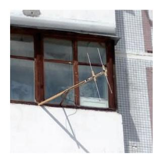
Design of the antenna is very simple. Personally I have made the antenna in 40 minutes. Antenna consists from reflector (length 1002-millimeters) and vibrator (length 972-millimeters, gap for coaxial cable- 10-millimeters). Distance between reflector and vibrator is approximately 204 – 210-millimeters.
