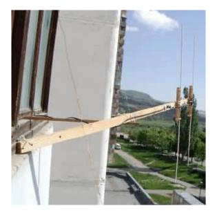
Antennas parts are made from insulated wire in diameter 4 millimeters. Place of vibrator, where a coax was installed, was protected with a raw compound. You may use another protector... SWR for the antenna (measured by SWR-121) was (1.0-1.1):1.
