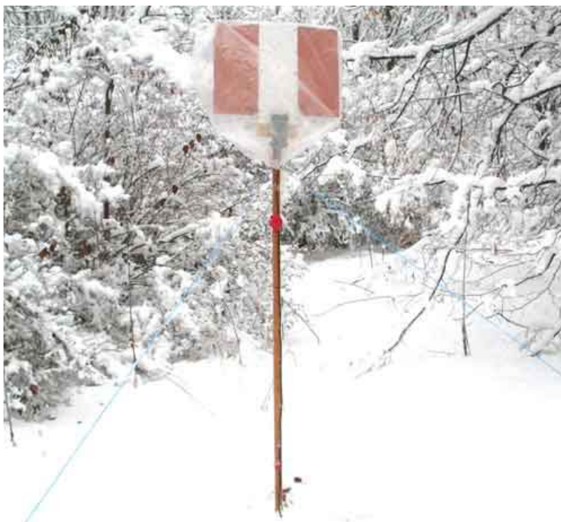
Figure 10 New Installed Flat – EH- Antenna
