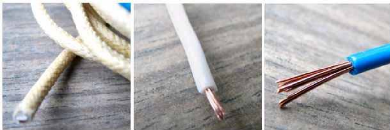
Photo 1 Examples of Some Good Antenna Wires
