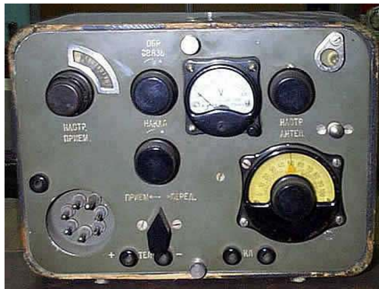
Russian Military/Spy/Partisan 3- tubes Transceiver "Sever." Regenerative RX + Xtall TX. Produced: 1940- 1945 Band: RX/TX: 3.62-12.25/3.62-6.25 Credit Line: http://www.cqham.ru/trx/sever.html
