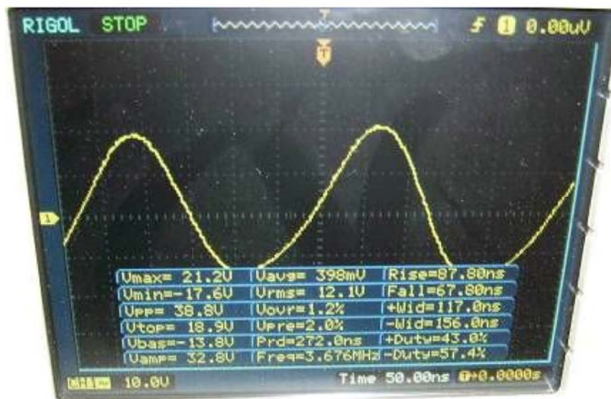
Figure 3 Output RF from the transceiver at TX- mode across a dummy load.
