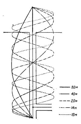
Figure 1 Current distribution along the antenna and the Stub
