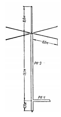
Figure 2 Design of the Vertical Antenna for 80-, 40-, 20-, 15- and 10- meter
