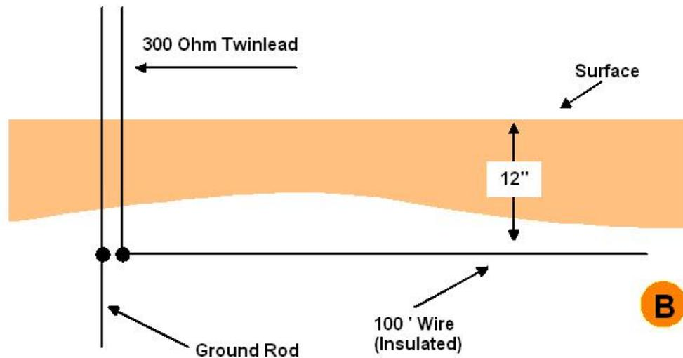
No surface, vertical 40 meter antenna was available to make signal comparisons but comparisons were made with a 40- meter dipole elevated about 40 feet. On local and short – skip contacts, the buried antenna was never better than 7 “S” units below the dipole with the average being 8-9 “S” units.
