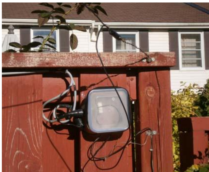
Picture 1 Feed Point of the Simple Broadband Antenna for the 40- meter Band
