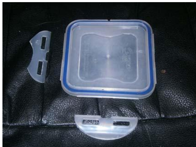
Picture 6 Cover with cracked retaining tags
