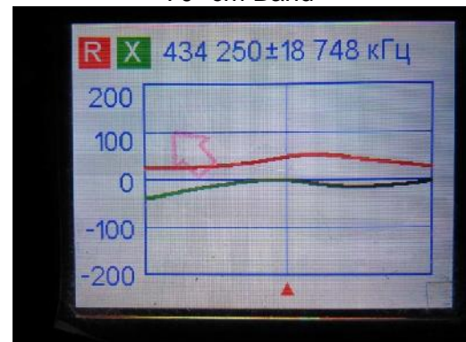
Figure 6 Z Vertical Antenna 5/8 Lambda for 70- cm Band
