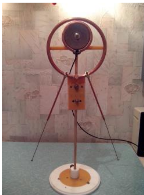
Figure 2 First Experimental Antenna made by R3PIN
