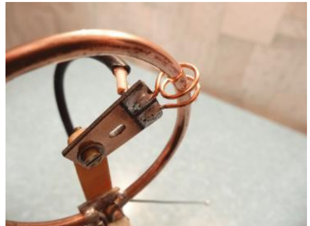
Figure 7 Fixture for Moving Coupling Loop
