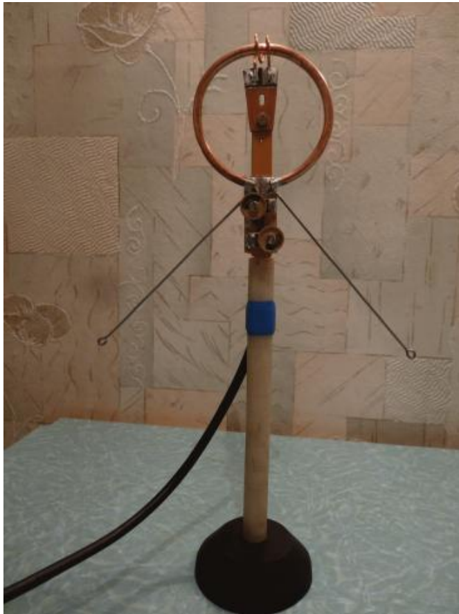
Figure 5 Small UA6AGW Antenna
