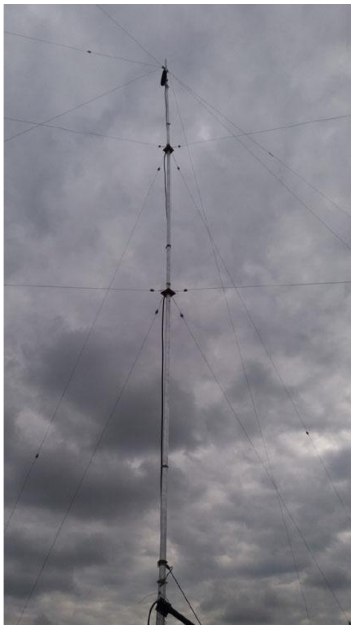
Inverted V Antenna for 80-, 40-, 30-, 20-, 15- and 10 meter Bands
