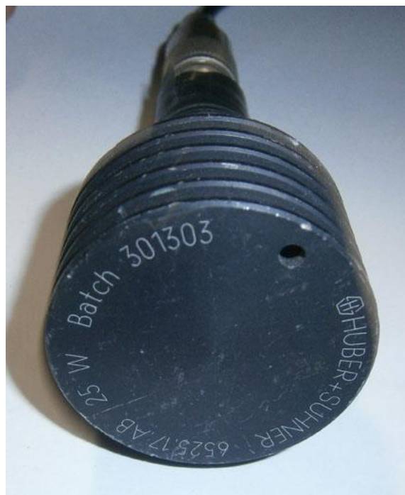
Photo 4 Huber + Suhner, 50- Ohm, 25 – Watt, 0- 2 GH Dummy Load
