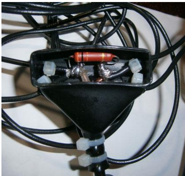
Photo 2 Cuplug before filling with epoxy
