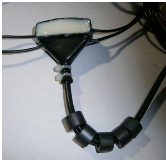
Photo 3 Ready Central insulator
