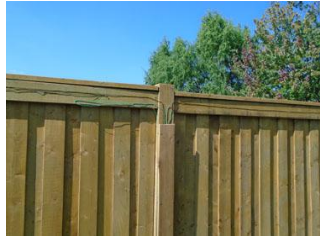
Low Profile Antenna for the 30, 20, 17, 15, 10 and 6- meter Bands Placed on a Fence
