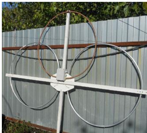
Figure 2 Design of the UA6AGW Balcony Antenna
