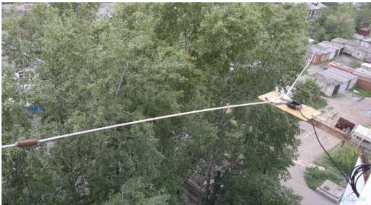
Figure 6 Dipole Antenna on the Balcony
