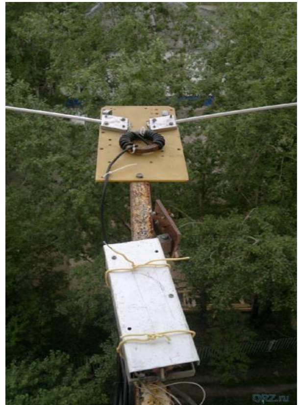
Figure 5 Dipole Antenna on the L-Bracket
