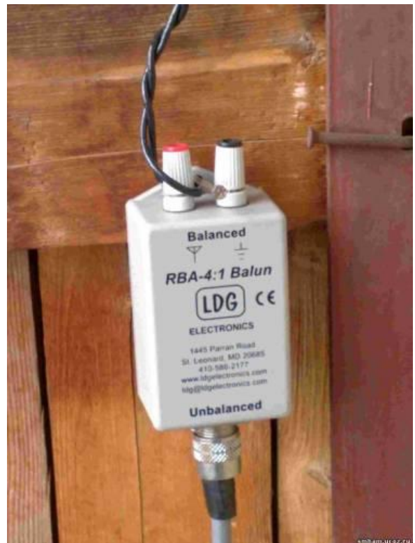
Picture 3 4:1 Balun from LDG Electronics at the Antenna
