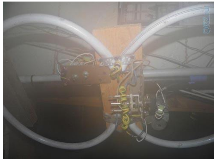
Picture 2 Simple Receiving Magnetic HF Antenna- S-Match Loop.
