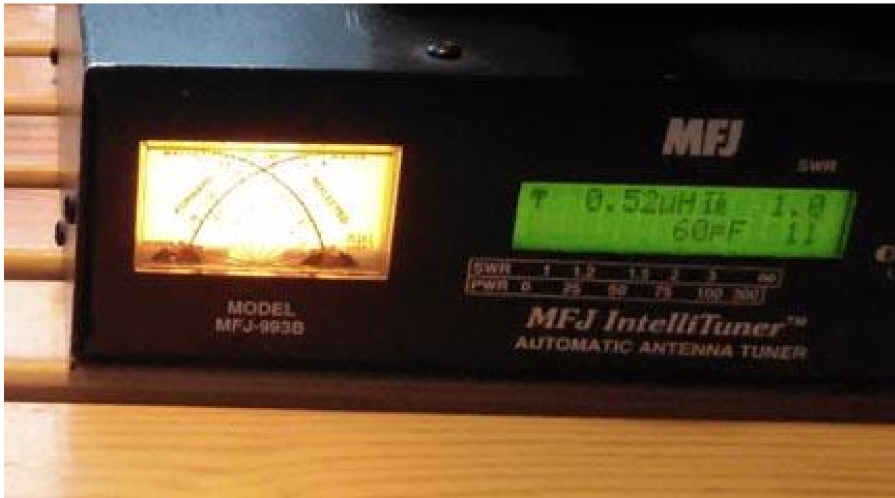
Picture 4 Value of the Matching L- Circuit on the 10- meter Band
