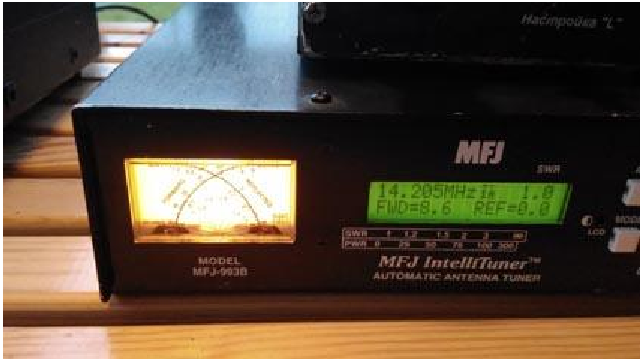
Picture 3 Reading of the MFJ- 993B on 20- meter Band
