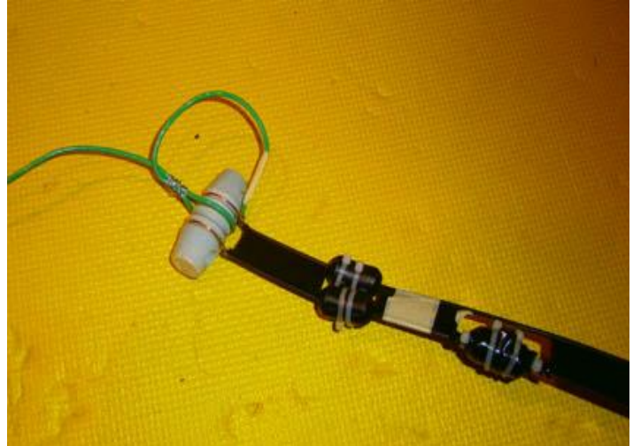
Photo 3 Antenna Wire Connection to the Two Wire Line
