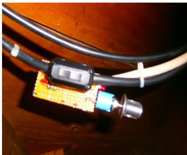
Figure 7 Glowing LED on the RF Current Sniffer with LED Indicator
