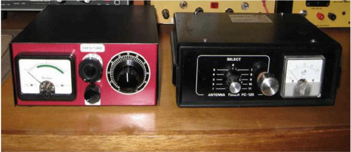
LHS of photo homebrew Earth Tuner and RHS modified commercial ATU to Ground Tuner.
