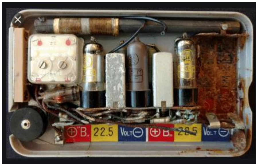
Ferrite Loop Antenna inside of a Tube Radio BAMBY from middle 1950'
