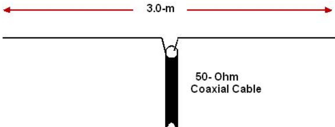
**Figure 1** Dipole Antenna for 6- meter Band
