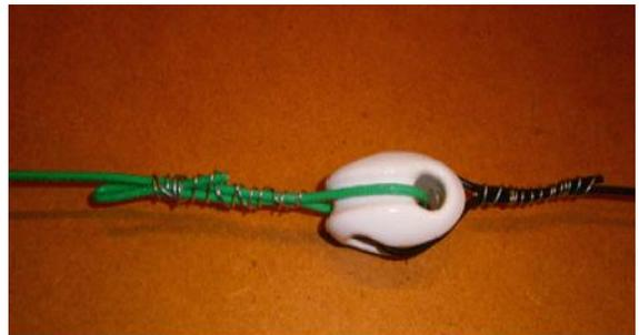
**Figure 4** Egg Insulator at the End of the Antenna
