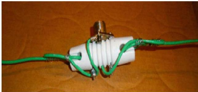
**Figure 3** Connector Mounted on Dog Bone Insulator and Antenna Wire Connected to SO- 239 Connector
