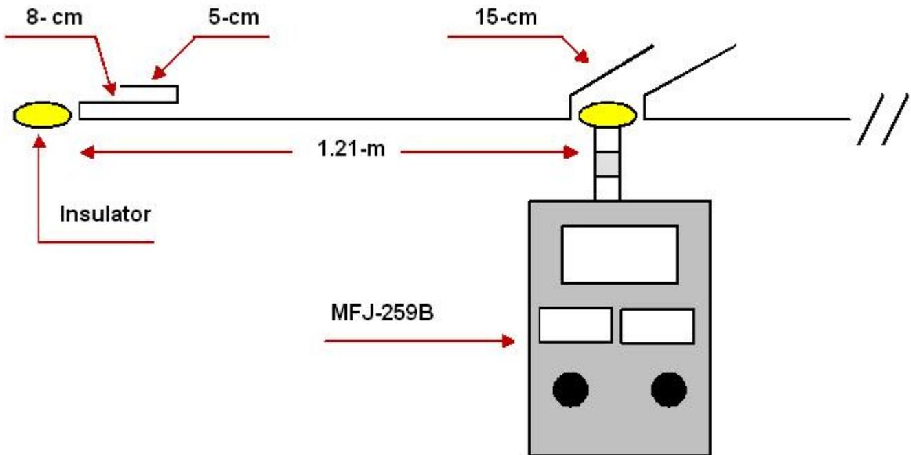
Figure 5 Dimensions of Antenna Tuned to 50.1- MHz
