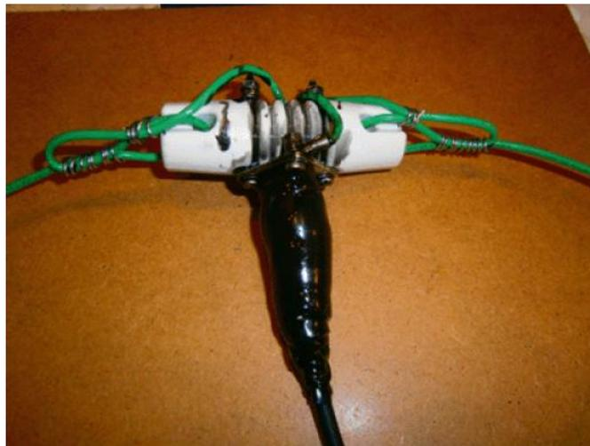
Figure 6 Center Insulator with Coaxial Cable
